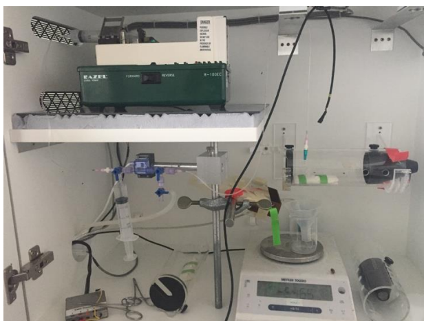
Figure 1: Cystometric recordings system. In the picture are represented the infusion pump, the pressure transducer, the scale, the restrained, the bladder infusion catheter, the electric wire to connect the electrodes and the amplifier.
